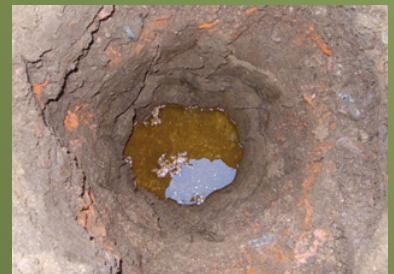
BOREHOLE SHOWING KEROSENE IN THE GROUNDWATER
