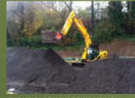
'TURNING' OF WINDROWS USING AN ALLU BUCKET
