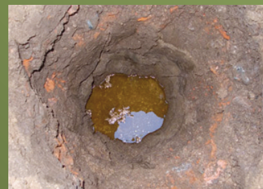
BOREHOLE SHOWING KERSENE IN THE GROUNDWATER
