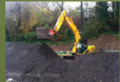
'TURNING' OF WINDROWS USING AN ALLU BUCKET
